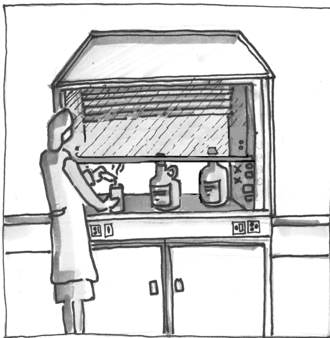
Handle highly toxic chemicals in a chemical fume hood.
